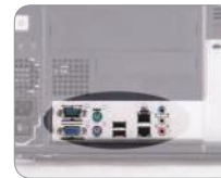
Front I/O design to facilitate ATE applications
