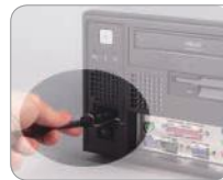
Plug ring-lock securely fastens the power cord
